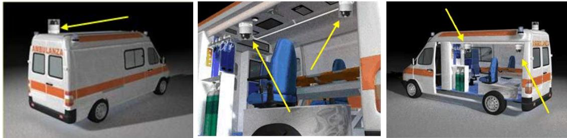
Fig. 3 – Location of video cameras on the mobile platform of MASMED system
