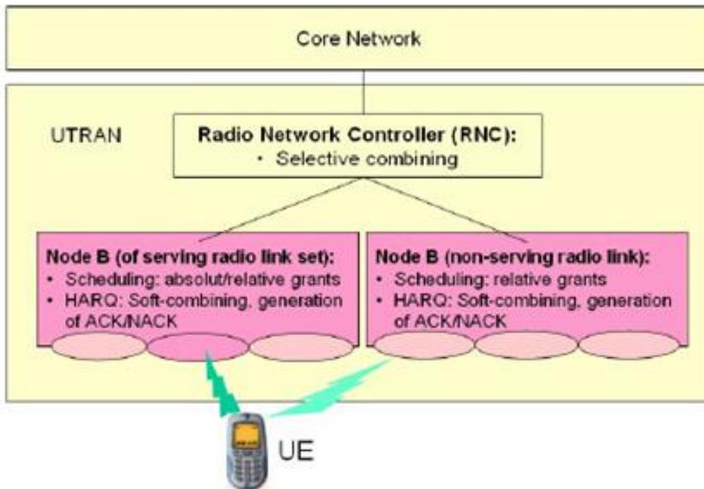
Fig. 4 – The programming mechanism and the HARQ protocol used by the HSUPA technology
